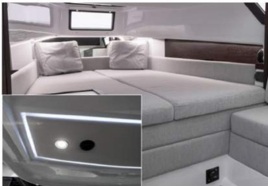
LED courtesy lights, front cabin and main cabin
